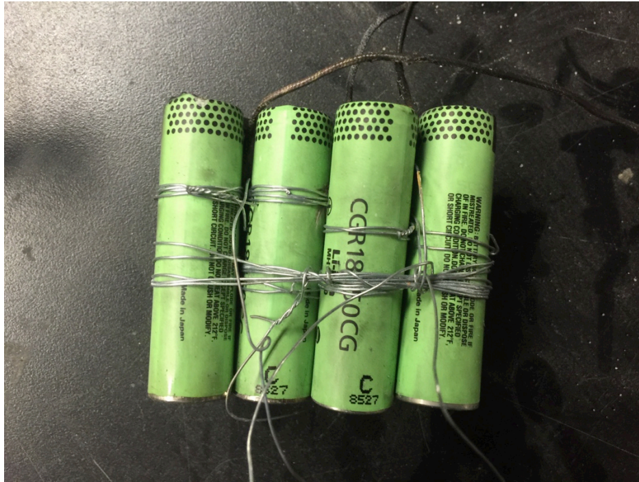
Figure 25 – Back side of Batteries After Immersion Testing
