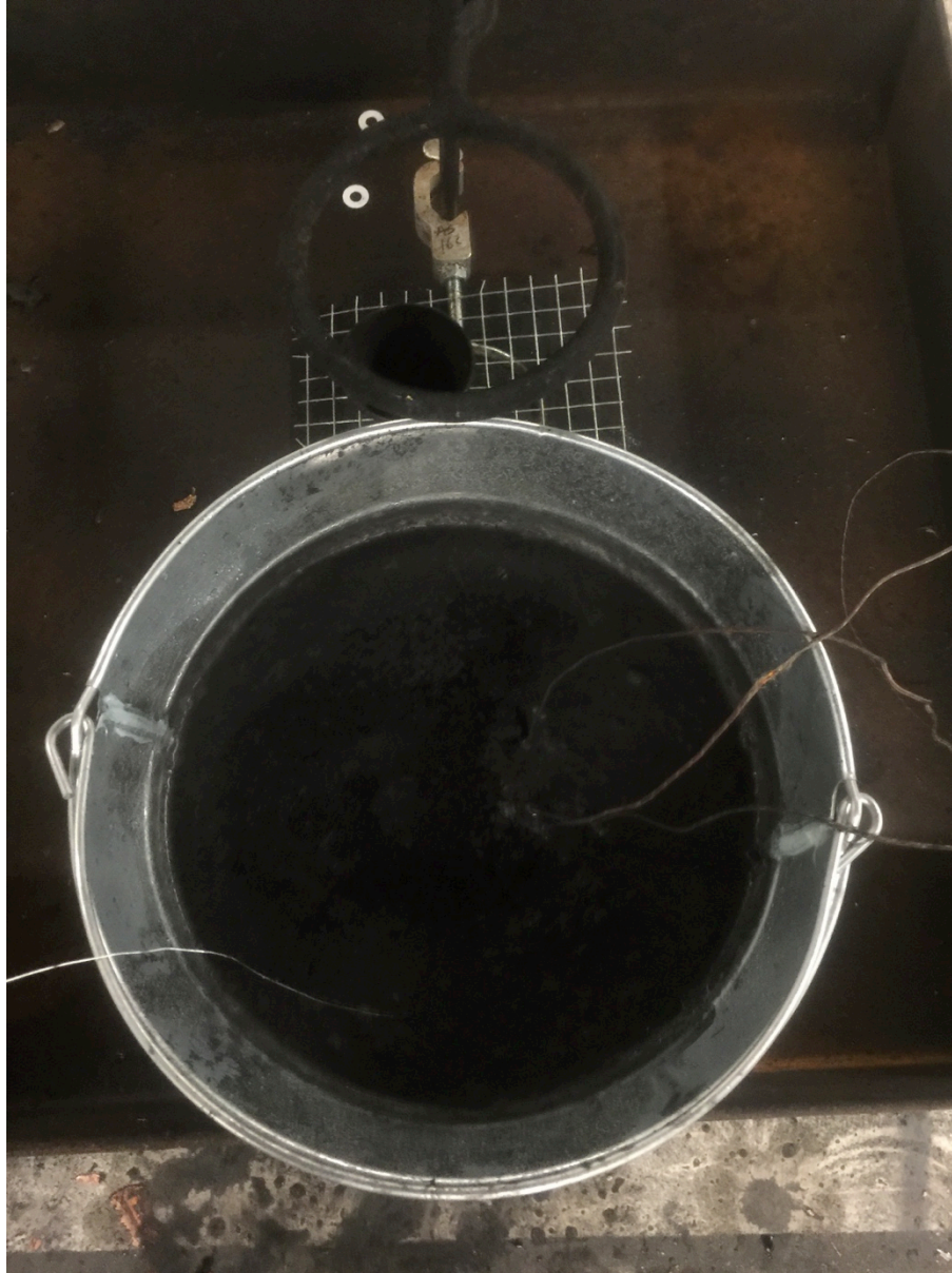
Figure 22 – Firelce After Battery Venting During Immersion
