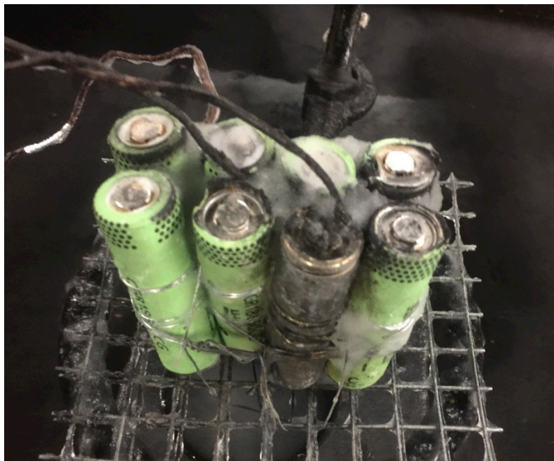
Figure 36 – FireIce Gel From Extinguisher Covering Batteries
