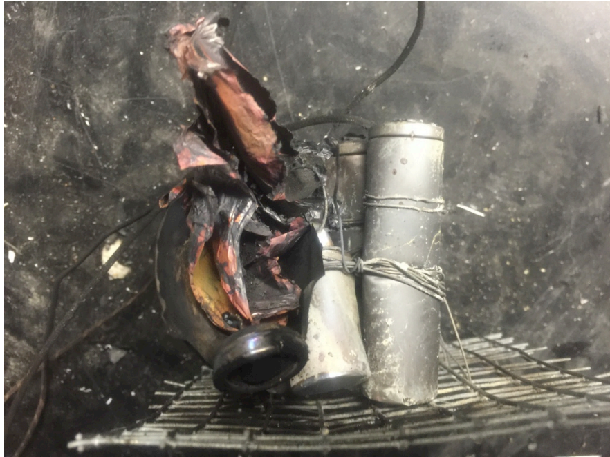
Figure 30 – Exploded Battery After Halon Extinguisher Test
