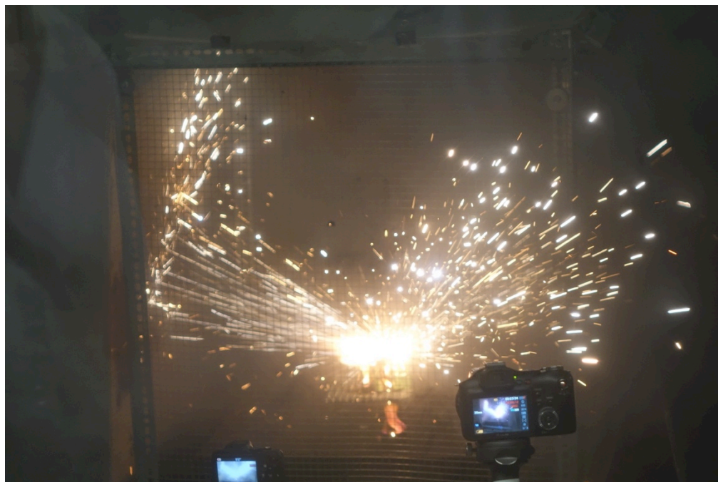
Figure 10 – Secondary Venting of Molten Material from Battery
