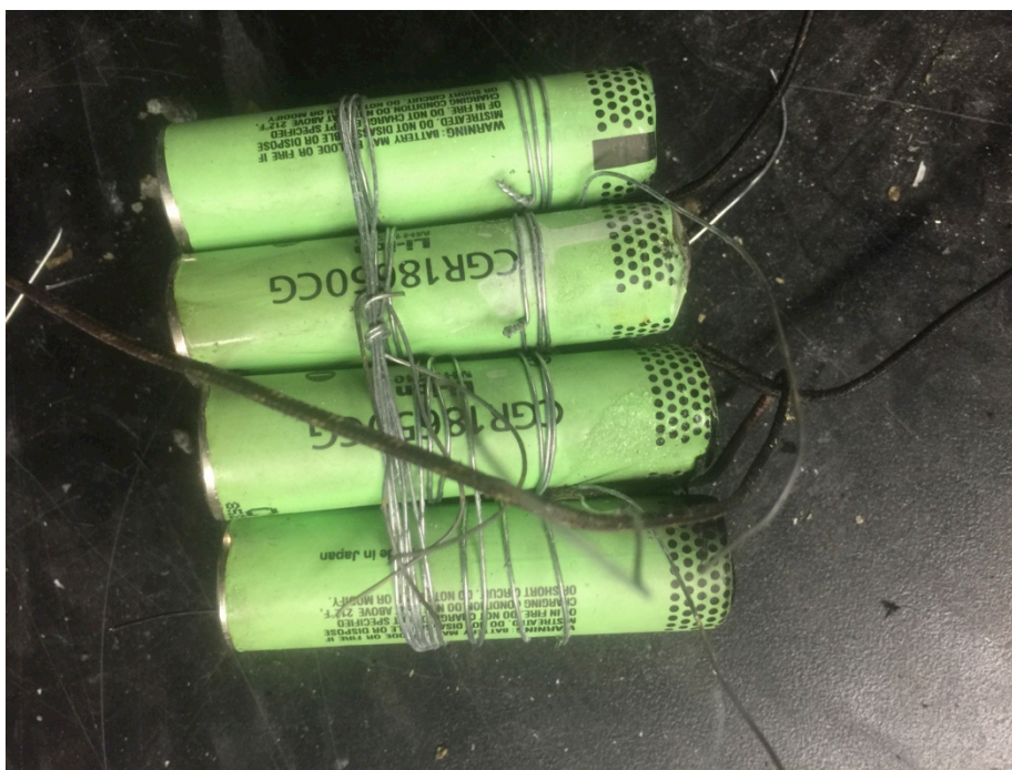
Figure 38 – Back Side of Batteries After Firelce Extinguisher Test
