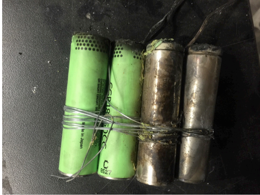
Figure 23 – Side of Batteries After Immersion Testing
