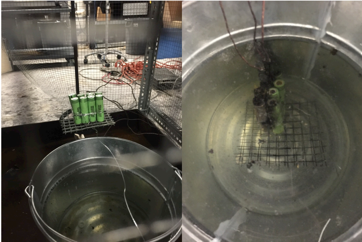
Figure 5 – Setup for Immersion Testing
