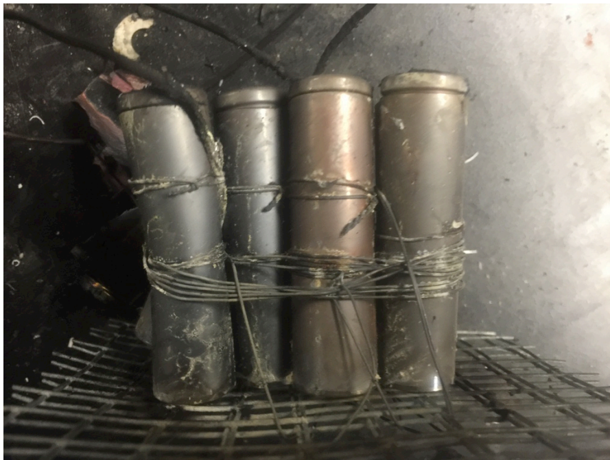
Figure 31 – Side of Batteries After Halon Extinguisher Test
