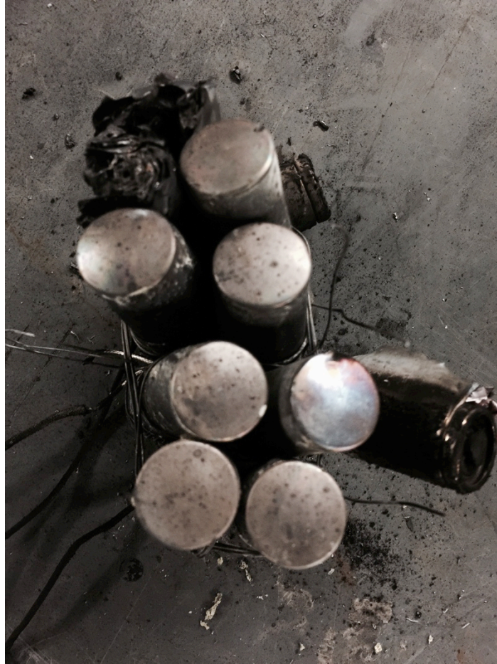
Figure 14 – Bottom of Batteries After Free Burn
