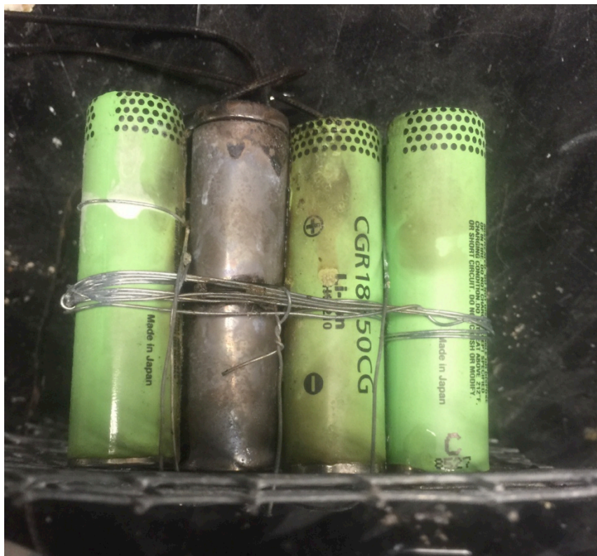
Figure 37 – Side of Batteries After Firelce Extinguisher Test
