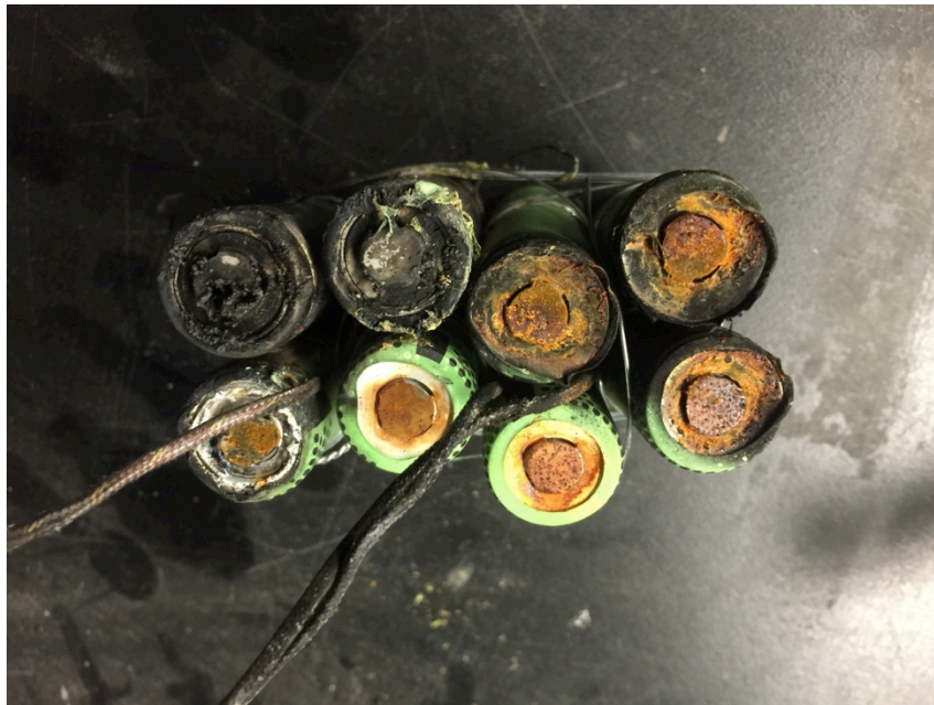
Figure 24 – Top of Batteries After Immersion Testing
