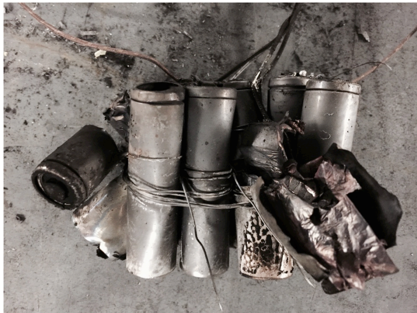
Figure 13 – Side of Batteries After Free Burn
