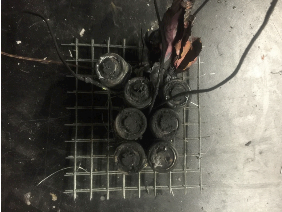
Figure 32 – Top of Batteries After Halon Extinguisher Test
