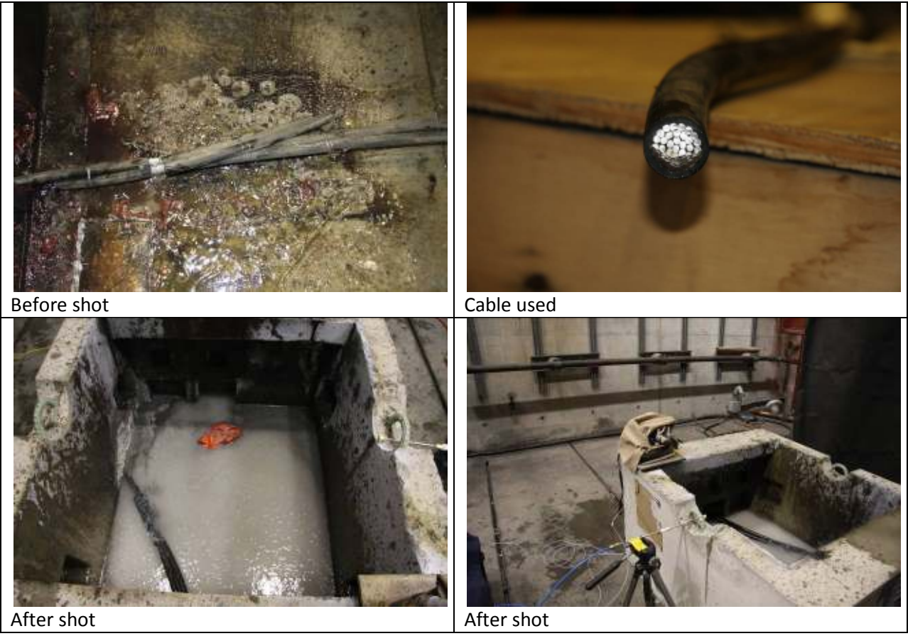
Figure 4 Cable Set-up Test # 4 and test outcome
